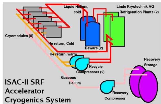
Figure 1: ISAC-II cryogenics system block diagram. Liquid Nitrogen delivery not shown.
