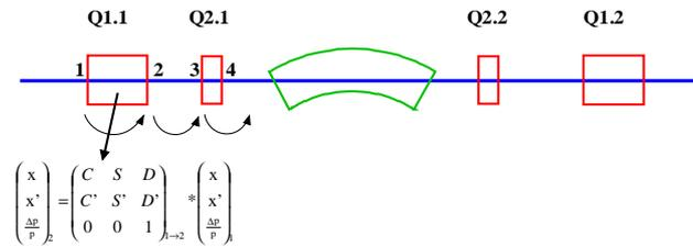
Figure 2: typical calculation scheme
