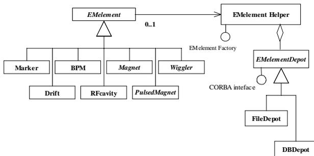
Figure 3: EMelement class diagram.
