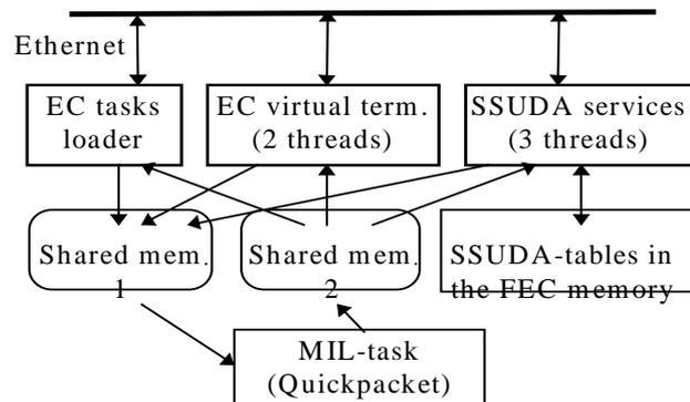
Figure 4 FEC software layout
