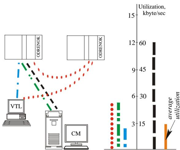
Figure 3: VEPP-4 control system intercomputer data flow and Ethernet capacity.
