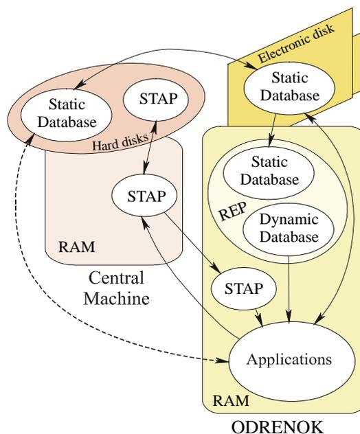
Figure 2: The VEPP-4 database arrangement.
