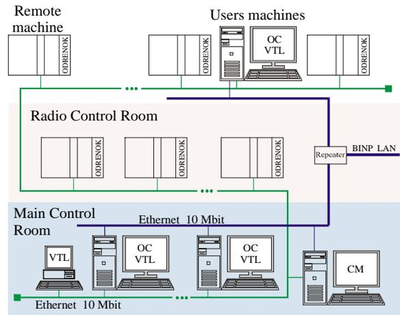
Figure 4: The second step of the VEPP-4 control system upgrade.
