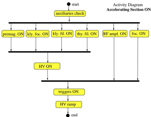
Figure 4: Activity diagram of the plant switching-on performed by the supervisor
