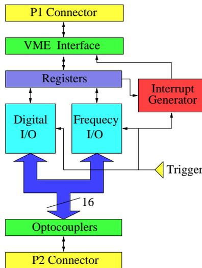
Figure 1: Multi I/O board block diagram
