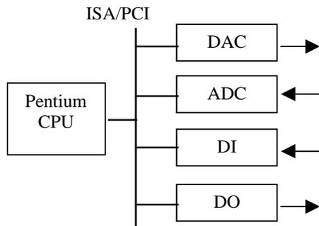
Fig.2 Front-end device controller structure
