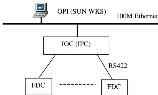
Fig 1 Structure of main PS control system
