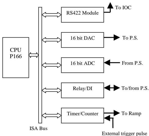
Fig 1. Front-end Device Control of Main P.S.
