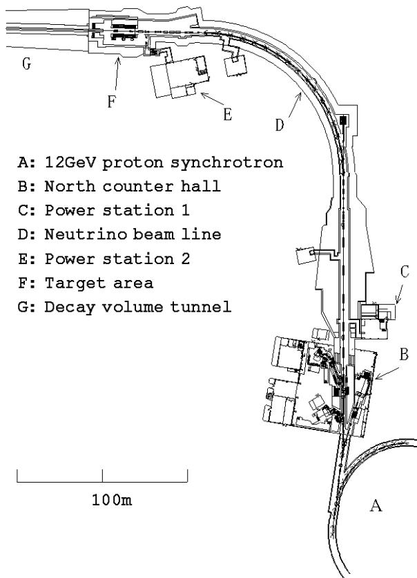
**Figure 1: 12GeV-PS, North counter hall, and neutrino beam line**
