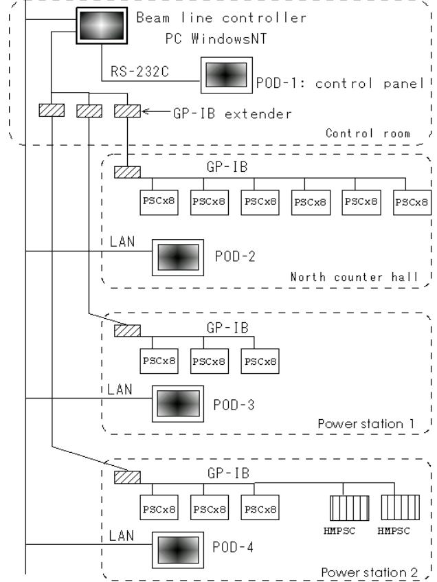
Figure 2: Configuration of control system
