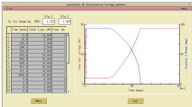
Figure 3: RF acceleration voltage ramping pattern editor window.
