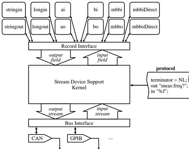
Figure 2: Interactions of the Stream Device Support [7].
