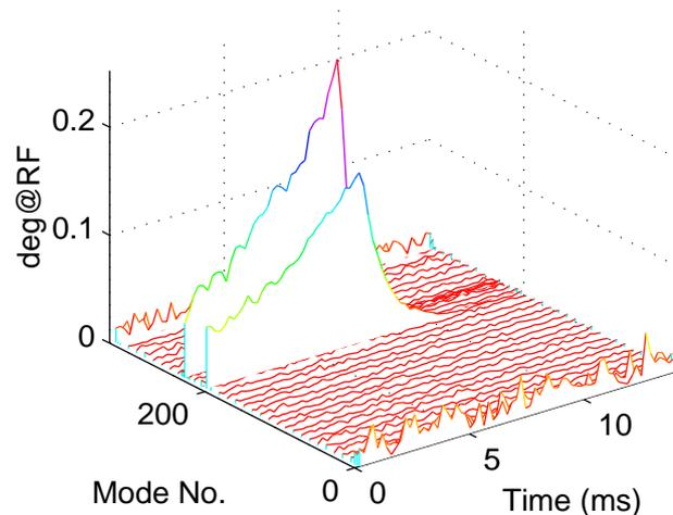
Figure 4: Bunch oscillation data transformed to modal domain shows modes 204 and 233
