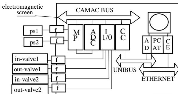
Figure 1. Fragment of hardware control system: MP-multiplexer; ADC-analog-to-digital converter; I-register; AD, CE-adapters; ps-pressure sensors; f-filters.
