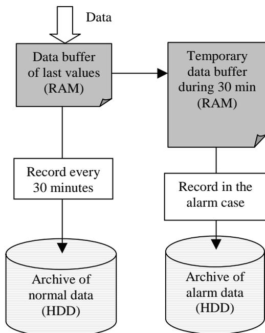
Figure 3: Mechanism of data recording.
