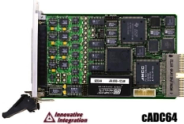
Figure 3: The CompactPCI I/O card, from Innovative Integration, with a TMSC32 DSP on board.
