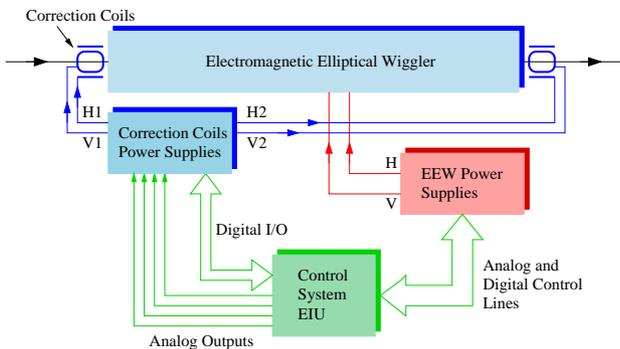
Figure 2: block diagram of the feed-forward correction system
