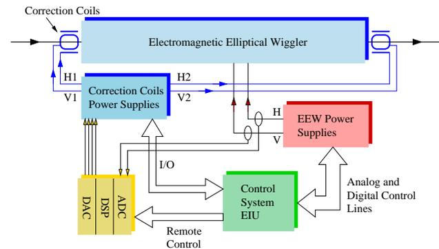
Figure 3: block diagram of the DSP-based correction system.
