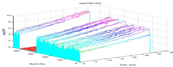
Figure 2:  $TM_{011}$  mode induced bunch oscillations.
