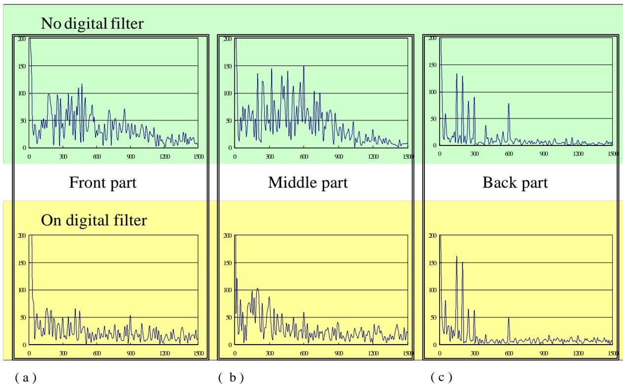
Fig. 4 Fourier analysis upper : without digital feedback of RQ lower : with digital feedback of RQ
