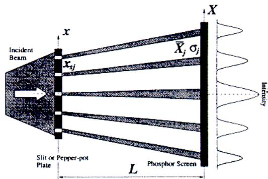
Figure 1: Typical setup for emittance measurement
