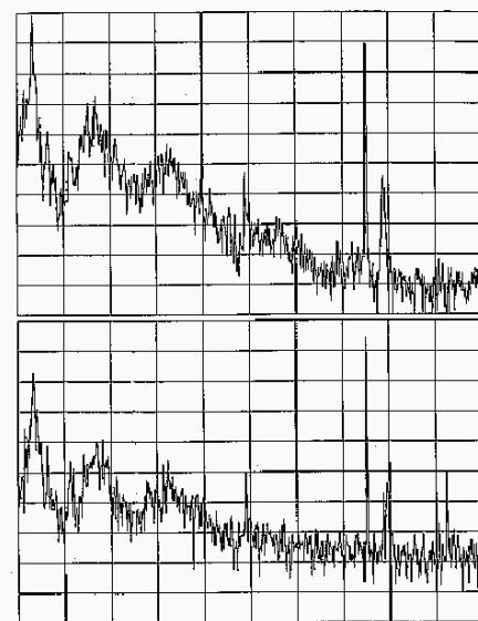
Figure 5: Spectrum of a dipole X ray beam position 25 m away from the source with feedback off and on (5dB/div, 200 Hz span).
