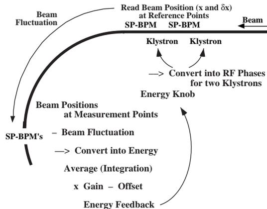
Figure 1: Process flow for beam-energy feedback.
