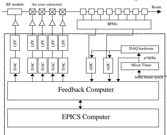
Figure 1. Fast feedback system schematic.
