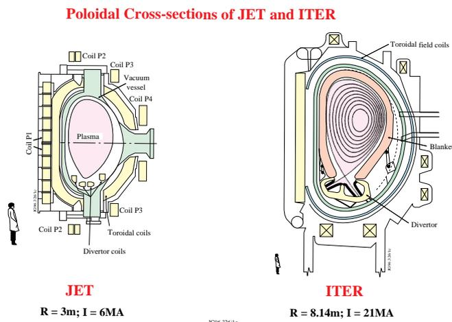
Figure 1 Cross sections of the JET tokamak and of the ITER reactor design
