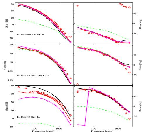
Figure 2 Measured (o) and modelled (lines) transfer functions between the PF coil voltages and plasma parameters.
