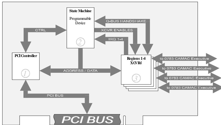
Figure 2. 0934 Module Block Diagram
