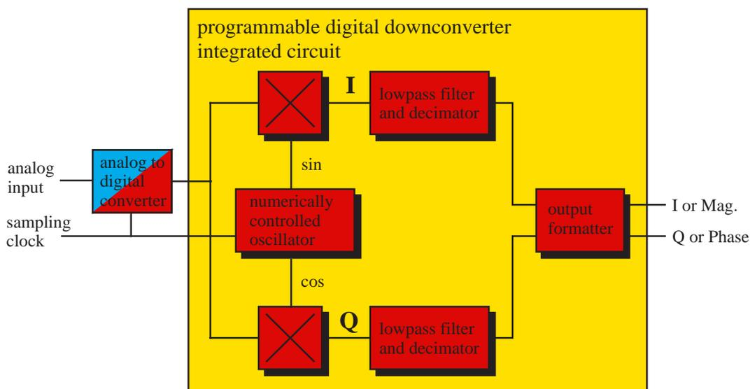
Figure 2: Functional block diagram of a DDC integrated circuit.
