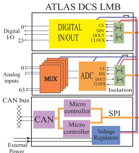
Figure 1 Block diagram of the LMB
