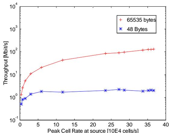
Figure 5: Throughput as a function of the Peak Cell Rate at the source (AAL-5, 155 Mbit/s link)
