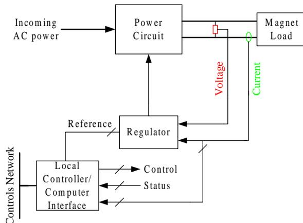
Figure 1: Generic Accelerator Magnet Power Supply
