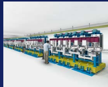
one BL consists of 18 in-vacuum undulators of 4.5m in length
