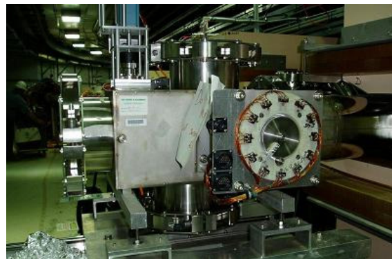
Figure 2: Primary stripper foil mechanism.
