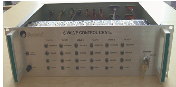
Figure 1: Six Valve Vacuum Control Crate.
