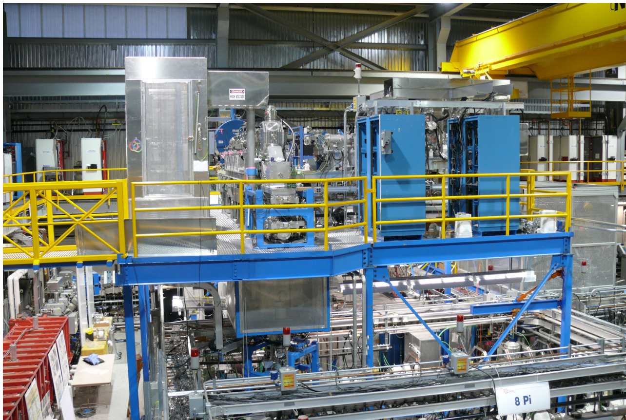
Figure 1: Picture of the TITAN platform. In the foreground one can see the vertical transfer beam line and the HV cage surrounding the RFQ cooler, in the background the circular shape of the MPET superconducting magnet. EBIT is behind the racks perpendicular to RFQ-MPET beam line.
