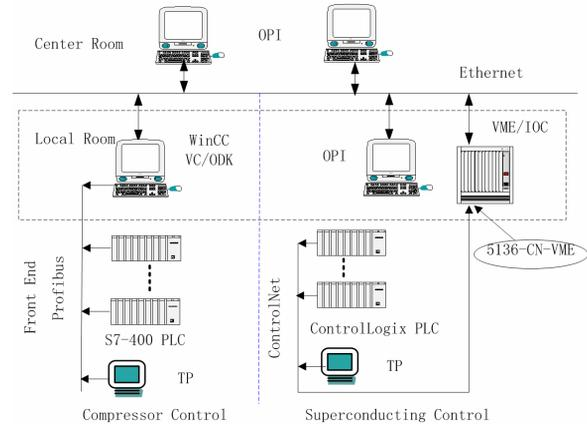
Figure 1: the cryogenic control structure of BEPCII project
