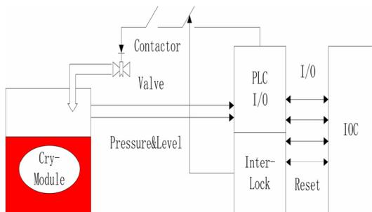
Figure 3: Design of Control Function of Superconducting Devices
