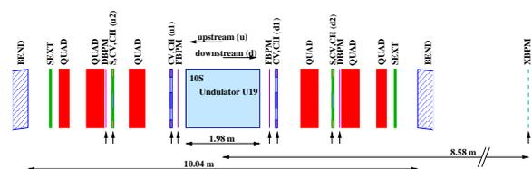
Figure 2: Layout of the 10S short straight section. The correctors and BPMs featuring in the correction procedure are indicated.
