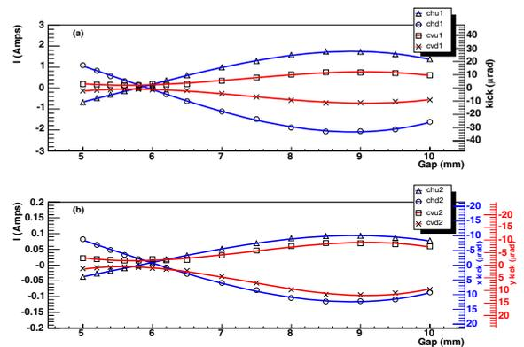
Figure 4: Corrected horizontal (red) and vertical (blue) currents and kick strengths versus gap for the (a) inner and (b) outer correctors (see Fig. 2). The various kick scales reflect the different corrector calibration constants.
