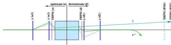
Figure 1: Electron beam trajectory through the insertion device and the emerging photon beam;  $\phi$  represents the deflection angles applied to the inner (u1, d1) and outer (u2, d2) correctors to counteract the ID edge kicks that result in the electron path displayed by the solid (green) line; the intended electron trajectory, after correction, is indicated by the dotted (green) line.
