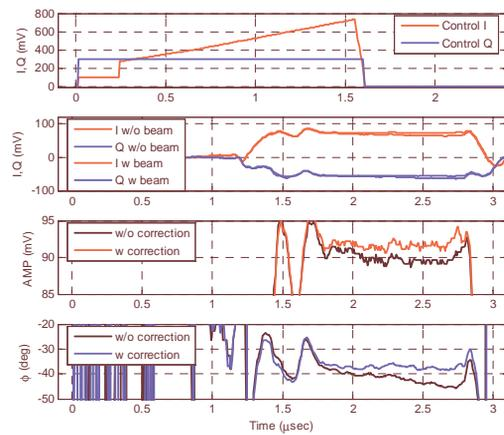
Figure 7: RF amplitude and phase waveform before and after correction with bunch train 600 nsec beam, both amplitude and phase are corrected simultaneously.
