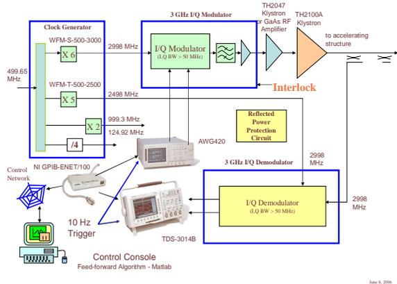
Figure 2: The block diagram of the updated low level RF system for the 50 MeV linear accelerator. It is a feed-forward enable system.
