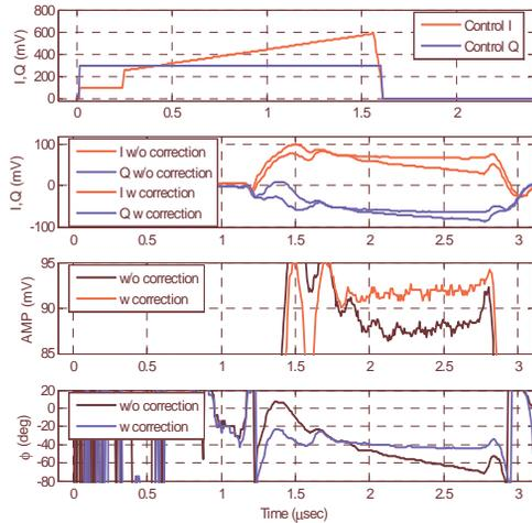
Figure 5: RF amplitude and phase waveform before and after correction I signal without beam, flatness of amplitude and phase are improved.
