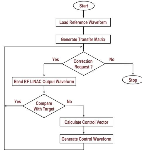
Figure 3: Flow chart of the feed-forward correction.
