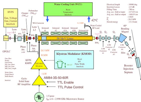
Figure 1: The synoptic of the 50 MeV linear accelerator system of the TLS.
