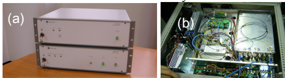
Figure 9: Exteriors of the 1550nm DFB laser source ((a), up side) and the optical comb generator ((a) lower side). (b) is the interior of the optical comb generator.
