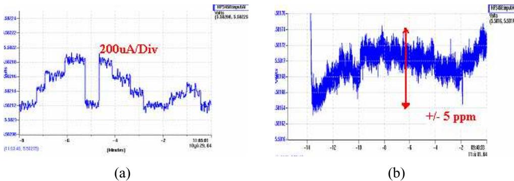
Figure 4: Output current measurement: (a) Step response at 55 Amps (200  $\mu A$  /Div)
