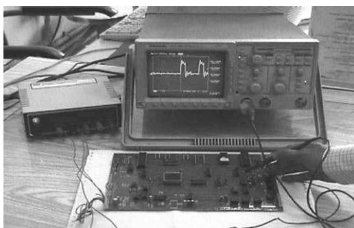
Fig3: Front Panel controller card under testing
