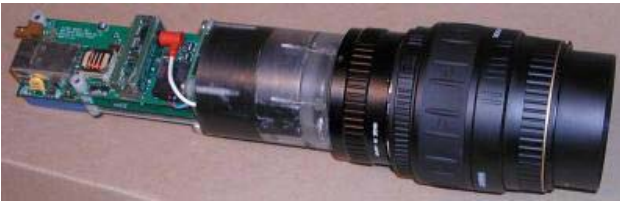
Figure 4: Camera assembly including CCD, acquisition, and networked computer
