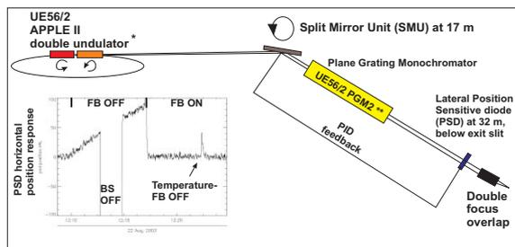
Figure 3: Prototype: horizontal mirror feedback[13].
