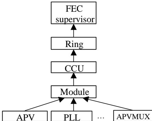
Figure 3: FEC electronics control hierarchy.
