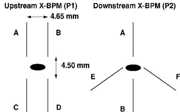
Figure 1. APS insertion device X-BPM geometry.
