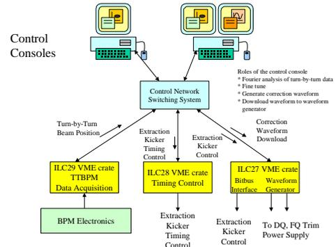
Figure 3. Tune acquisition and correction system.
