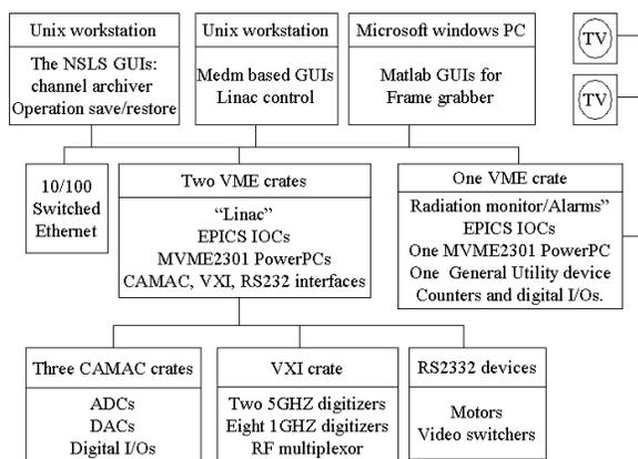
Figure 1: The Hardware/software Illustration of SDL Control System
