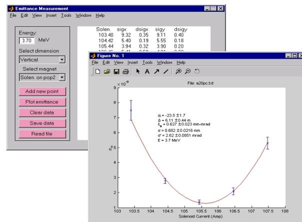
Figure 4: Automated emittance measurement using Matlab and Epics.
