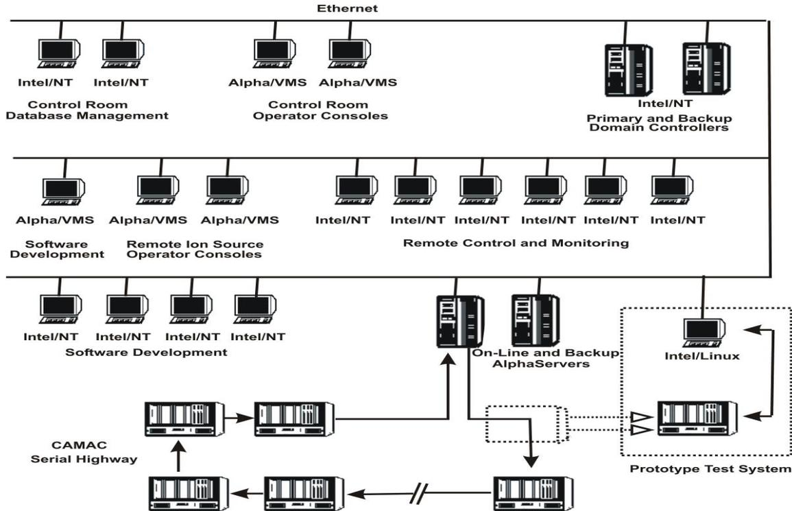
Figure 1: ATLAS Control System Showing Prototype Distributed I/O
