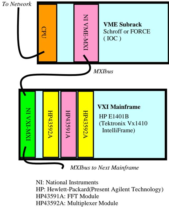
Fig. 1. Basic system configuration of a BM IOC.
