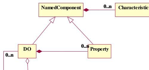
Figure 1: DO – Property – Characteristic class diagram
