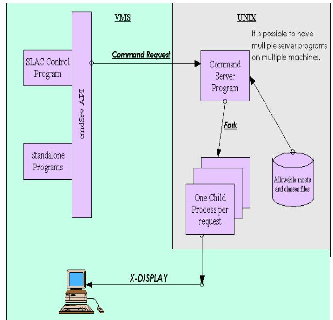
Figure 2.1: Simple cmdSrv Example Configuration
