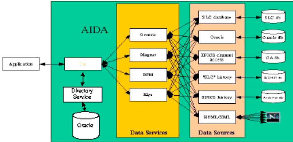
Figure 2: Logical Architecture, showing get/set/monitor, to/from any data source through a data service
