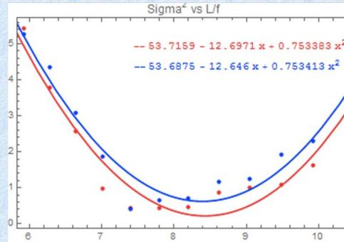
The horizontal axis shows ratio of distance from the solenoid center to the profile monitor and solenoid's focal length. Vertical axis shows the square of the r.m.s. beam size in mm<sup>2</sup>. The maximal difference between the parabolic fit coefficients is 0.2%. Distance from the solenoid to the profile monitor is 3.63 m. Emittance for the blue curve is 0.19 mm mrad, and for the red curve it is 0.11 mm mrad, difference is factor of 2.
