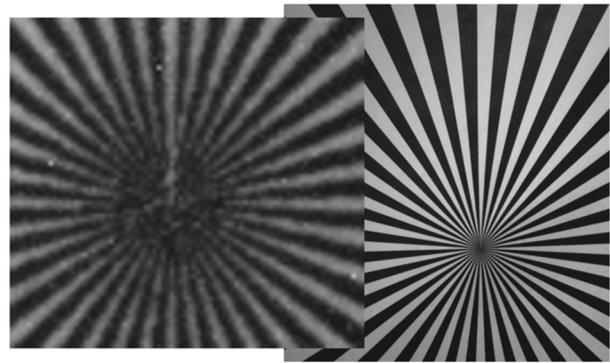
Figure 4: The Camera image after 1800 MWhrs of exposure at 1.4 MW at 1 GeV. Left a close-up of the test image center.
