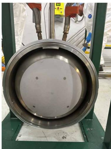
Figure 6: Fiducial markers on the vacuum window.
