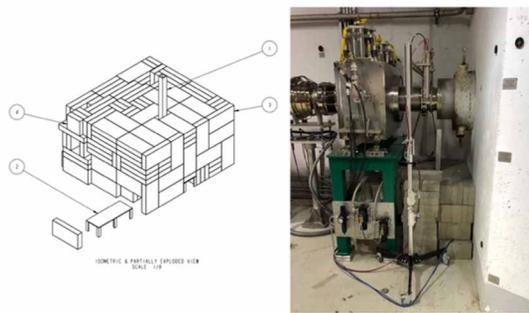
Figure 2: The shielding blocks to protect the camera.
