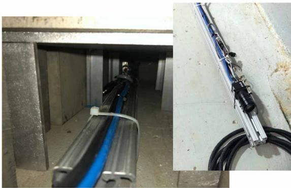
Figure 3: The camera inserted into the shielding blocks arrangement.
