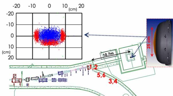
Figure 1: The Ring Injection Dump line along with the calculated projection of beam particles on dump window.
